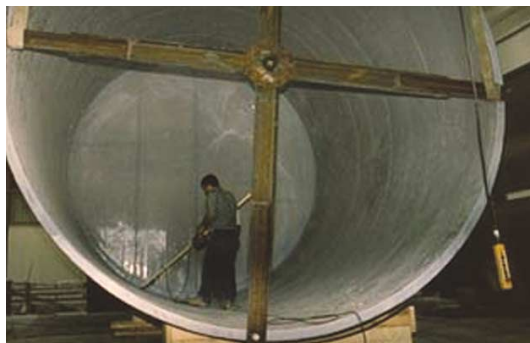
C.P.F. Dualam used dualam technology to fabricate this FRP chlorine neutralization tank with DERA KANE* MOMENTUM* 441-400 Epoxy Vinyl Ester Resin.
